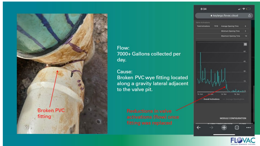
Figure 1 Identification of Infiltration
