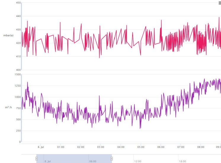
Figure 13 Set point vacuum level (mbar) vs. Air Flow (m 3 /h) indicating system performance and condition.
