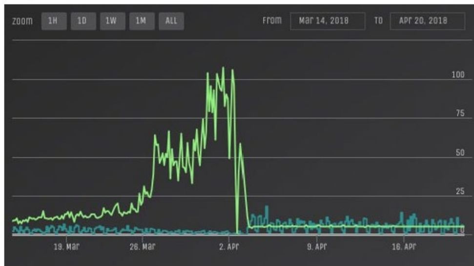
Figure 27 Graph depicting failing valve controller.
