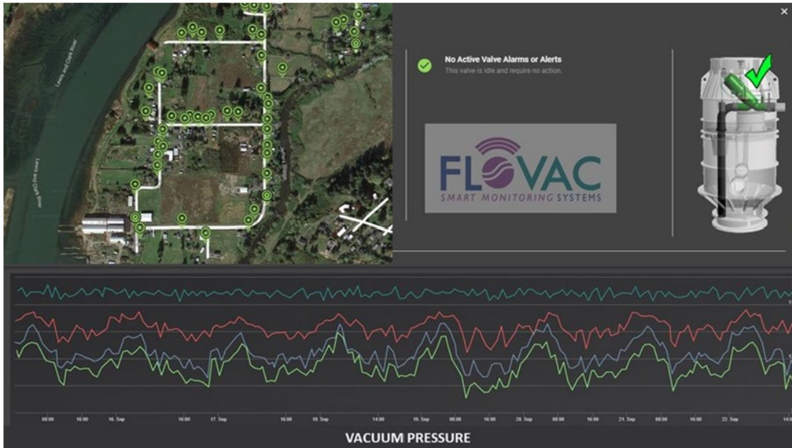
Figure 29 Brief overview of FMS interface with vacuum measurements.
