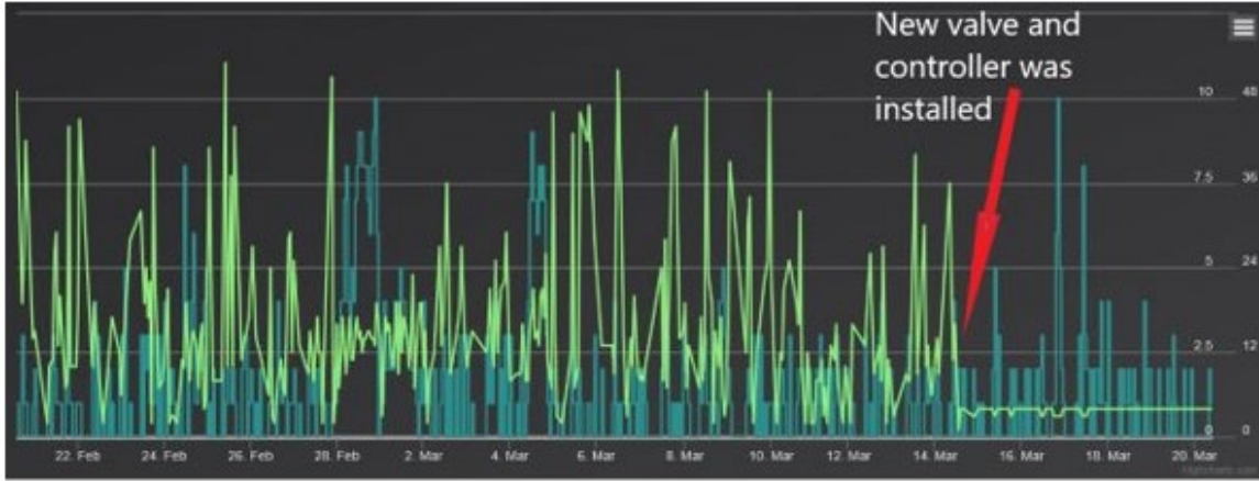
Figure 28 Erratic timing of HP controller replace with Flovac Controller
