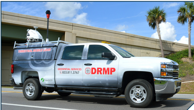
The DRMP Mobile LiDAR Truck
