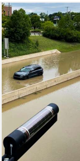
A Hyfi sensor watches a flooded Dearborn underpass, driving road-closure calls.
