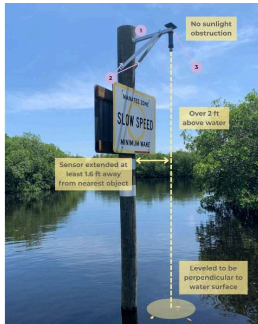
Installation guidance: over-water monitoring.
