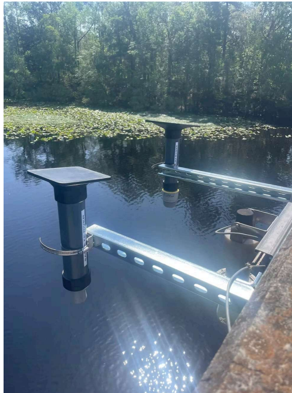
Ultrasonic and radar stations deployed side by side.
