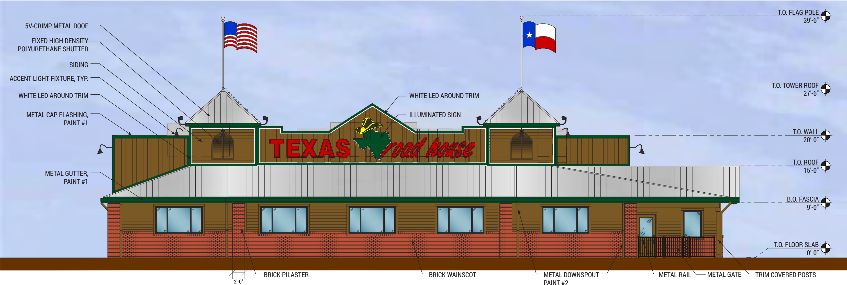
FRONT ELEVATION (SOUTH WEST)
