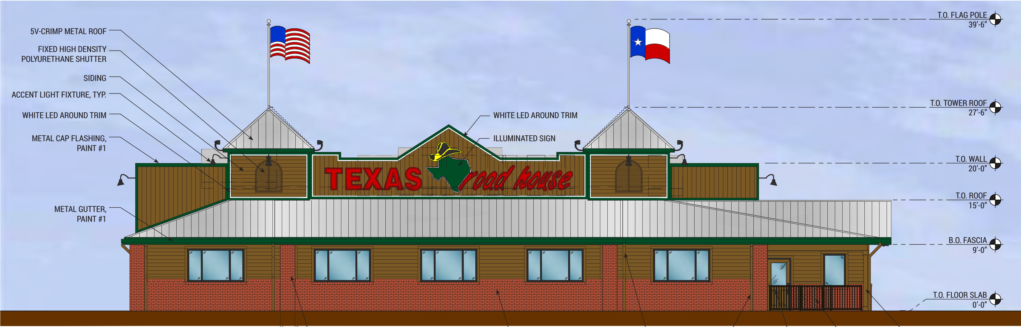
FRONT ELEVATION (SOUTH WEST)
