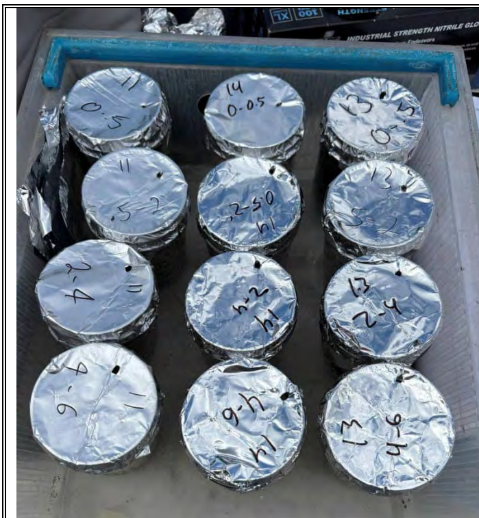
Photo 17: Soil samples collected for OVA screening and lithology description.
