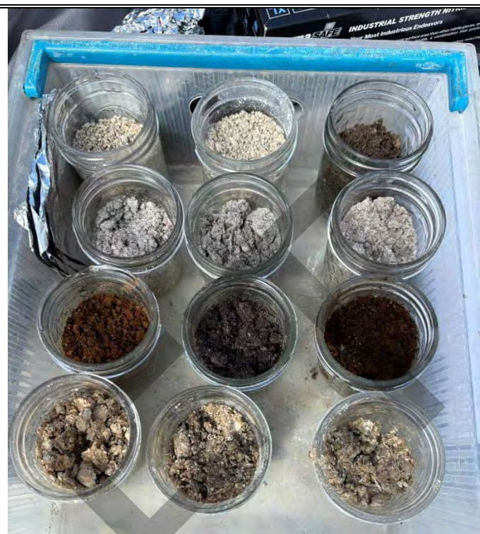
Photo 18: Soil samples collected for OVA screening and lithology description.
