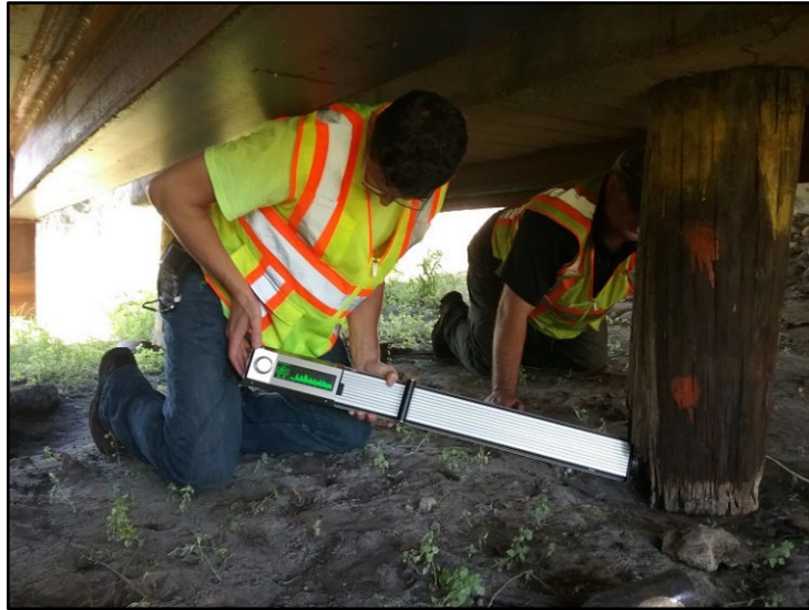
Drill Resistance Device Testing Bridge Piles, Collier County, FL
